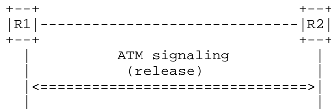
(b) Flow ID removal through ATM signaling
