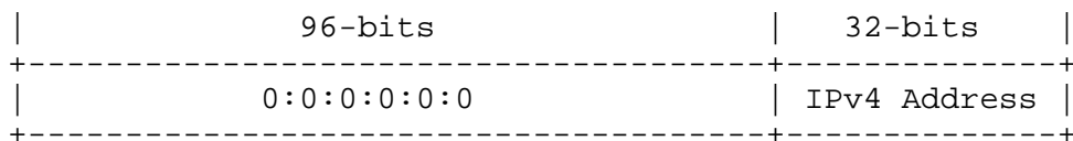
IPv4-Compatible IPv6 Address Format
